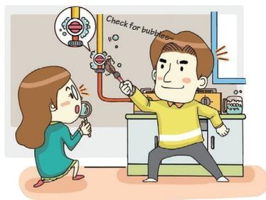
\* Check the hose and the joint between the hose and gas burner using soap water or inspection fluid.
